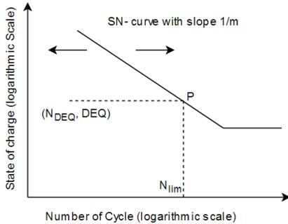
Fig. 2. S-N curve for a battery.
